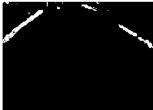
Step 4: Thresholded final image of lane lines
